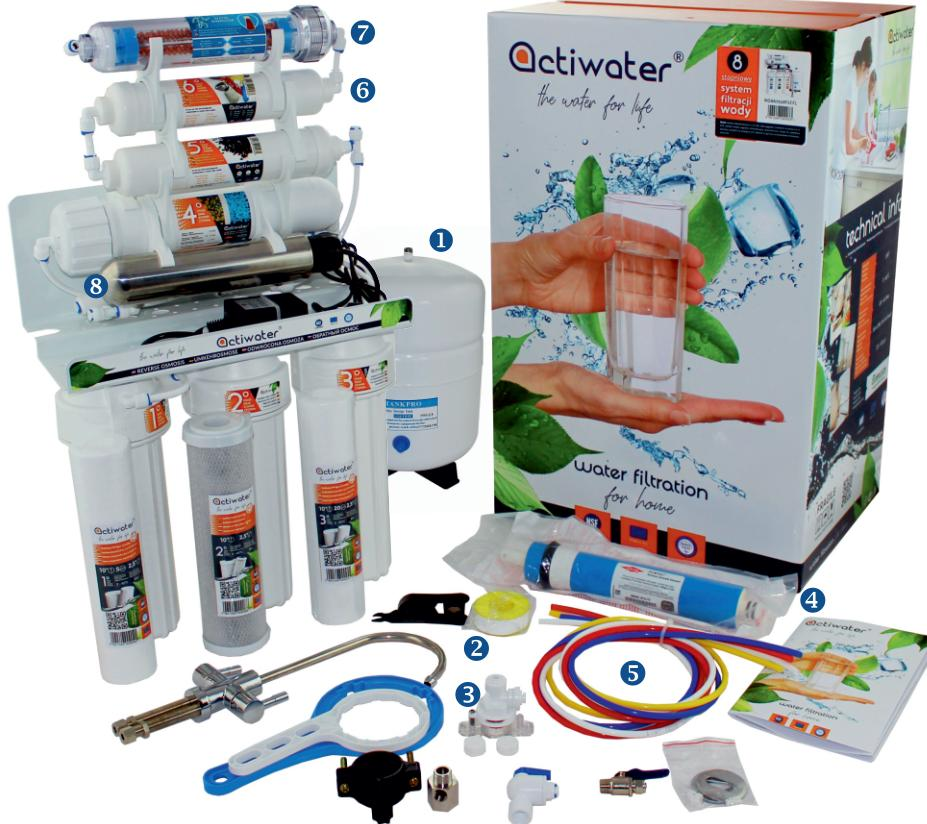
**SET ELEMENTS:** sediment filters 5 i 20 micr., carbon block, RO membrane: 100 GPD, inline carbon filter - coconut carbon media mineralizing filter, bioceramic filter, UV lamp, double faucet, tube - 1/4", 3/8" connection, 2,8 gal metal tank wrenches for membrane housing and filter housings.
